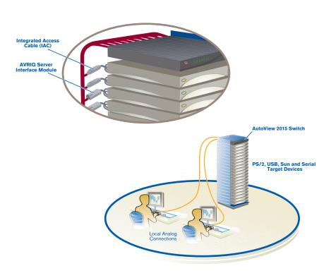
The AutoView switching solution provides support for USB and/or PS/2 user keyboards and mice and USB, PS/2, Sun or serial target devices in a single solution.
