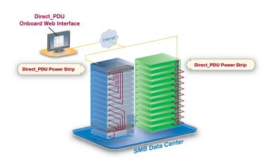
The Direct\_PDU power strip includes a built-in Web interface for easy, remote access and control.
