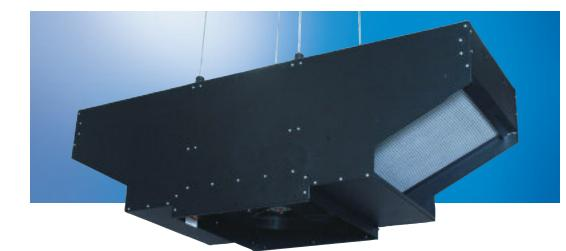
The ceiling mounted Liebert XDO overhead cooling module provides sensible spot and zone cooling for high heat density equipment. The Liebert XDO draws in hot air through two opposite inlets and discharges cool air down into the cold aisle where the electronic equipment air inlets are located. This flexible, scalable and space saving product mounts to the ceiling — requiring zero floor space.
