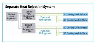
The indoor Liebert XDC Refrigerant Chiller is specifically designed to support Liebert XD cooling modules. Liebert connects directly to the modules through the pumped refrigerant circuit.
