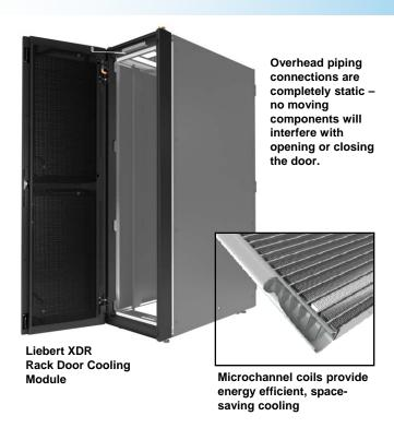
The Liebert XDR is a fanless heat exchanger module that installs as the rear door of an equipment rack, providing up to 20kW of roomneutral cooling. The Liebert XDR design uses the server fans within the protected rack to provide airflow through the unit. The microchannel coil heat exchanger cools the air and returns it to room at close to the same temperature as the air entering the rack.
