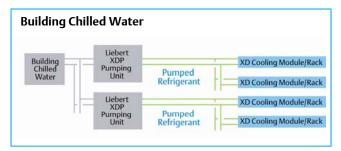
When a building chilled water circuit is available, the Liebert XDP Pumping Unit is utilized as an interface between the pumped refrigerant circuit and the chilled water system. Both Liebert XDC and Liebert XDP units circulate the refrigerant to the Liebert XD modules, while maintaining the refrigerant at a temperature always above the actual dewpoint.
