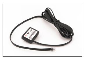
The R170 PDU Sensor Tag is ideal for data center managers that want to minimize wiring and eliminate the costly administrative overhead of managing IP connections to each PDU.
