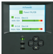
Individual current measurement for each fuse/breaker
