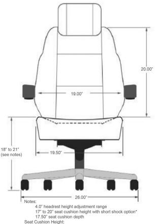
Regular Shock Option - Seat Cushion Height 18" to 21" Short Shock Option - Seat Cushion Height 17" to 20" Tall Shock Option - Seat Cushion Height 19" to 23"
