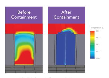
CFD analysis shows a significant reduction in hot air recirculation when Sliding Doors are applied in conjunction with Rack Top Baffles at the end of the cold aisle.
